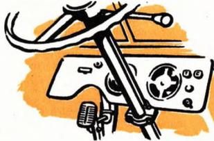
Electric starter button on instrument panel provides new, clear floor area while Chevrolet's new solenoid-operated mechanism assures positive starting.
